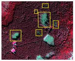
This series of pictures shows an example of the possible development of detected beetle nests: At the beginning of the season in May, two beetle nests were detected. In June, the infested trees have already been removed. Over the course of the season, the further gradual spread of the beetle is clearly visible.
